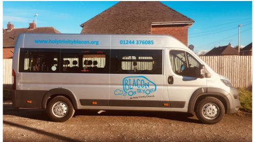
Our minibus has 16 passenger seats. It has a lift to enable a wheelchair to be lifted on board: with one wheelchair there would be room for 10 other passengers.
